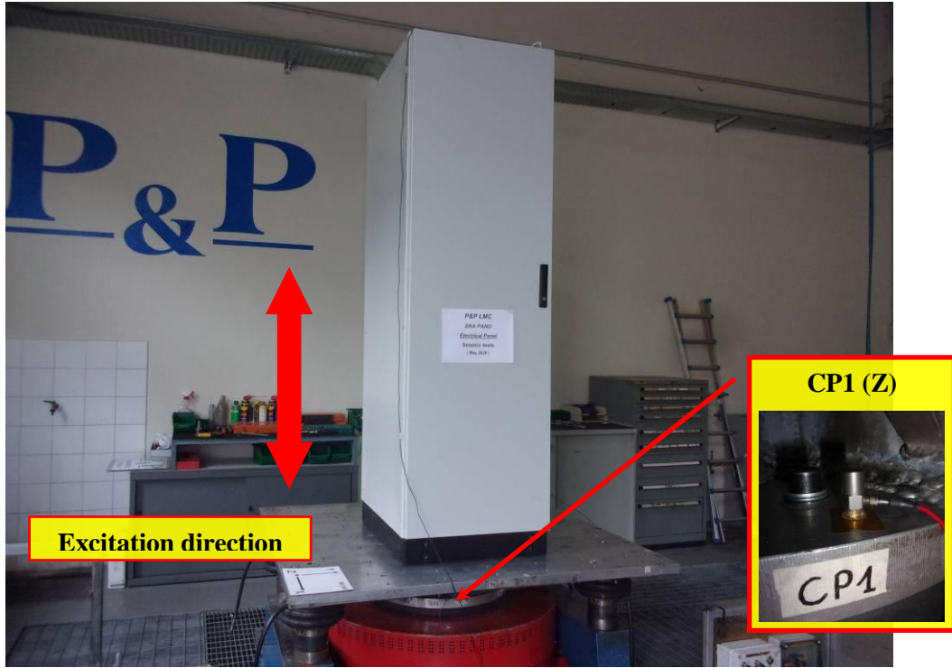
Photo 3: Test configuration for seismic test in Z direction
