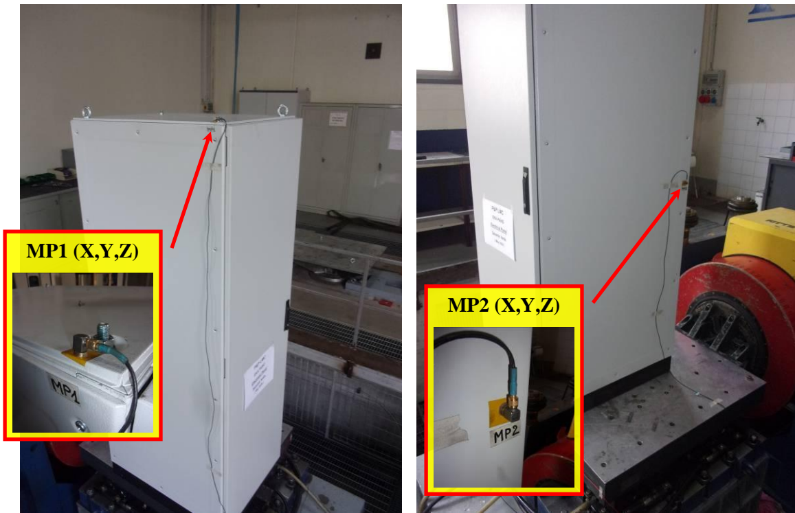
Photo 4: Measuring accelerometers MP1 and MP2
